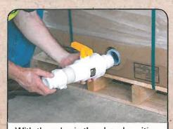
With the valve in the closed position, begin threading the ball valve assembly into the dispense gland. (Note, here a quick connect has been attached to the outlet of the valve.)
