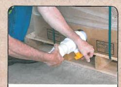
As the assembly is threaded into the dispense gland, the nipple will push the crown cutter forward piercing the inside liner membrane.
